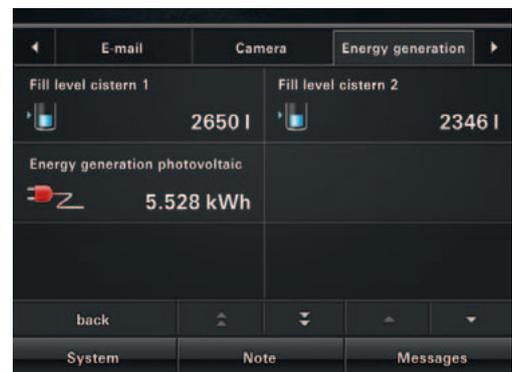
The water level of a cistern or the energy generation of a photovoltaic system can be viewed via the Gira Interface.
