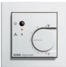
The automatic regulation of humidity ensures that ventilation is only switched on if the humidity exceeds a preset value. The humidity is recorded using sensors, and if the desired value is exceeded, a connected fan is switched on for dehumidifying. Thus, unnecessary ventilation and the consequential loss of valuable heat are prevented. In addition, counteracting increased humidity guarantees a comfortable and healthy room climate and prevents the damaging growth of mould.
