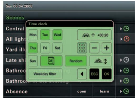
A separate user profile can be created for each individual room with times in which the room should be heated or ventilated. This means that heating and ventilation systems never run unnecessarily.
