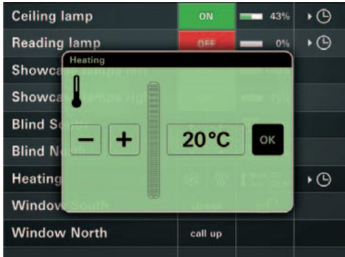
The temperature can be controlled conveniently and individually for each room. The system registers by means of door and window contacts when a door or window is opened and lowers the heating.
