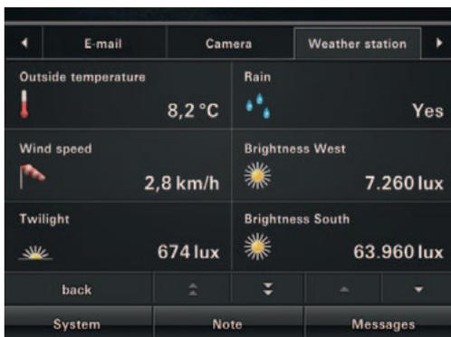
The data from a weather station can be viewed. The weather station measures wind speed, precipitation, twilight, temperature and brightness.
