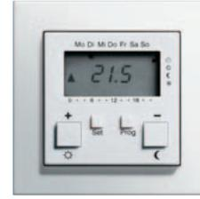
The connection to a seven-day time clock allows a great deal of need-based control of heating and cooling. Switching points which can be distributed during the week can be set up to adapt the temperature control of the rooms exactly to the weekly schedule of the users. If the rooms are unused, unnecessary heating is prevented. In addition, this heating optimisation offers comfort and savings and ensures that the desired temperature is reached on time.
